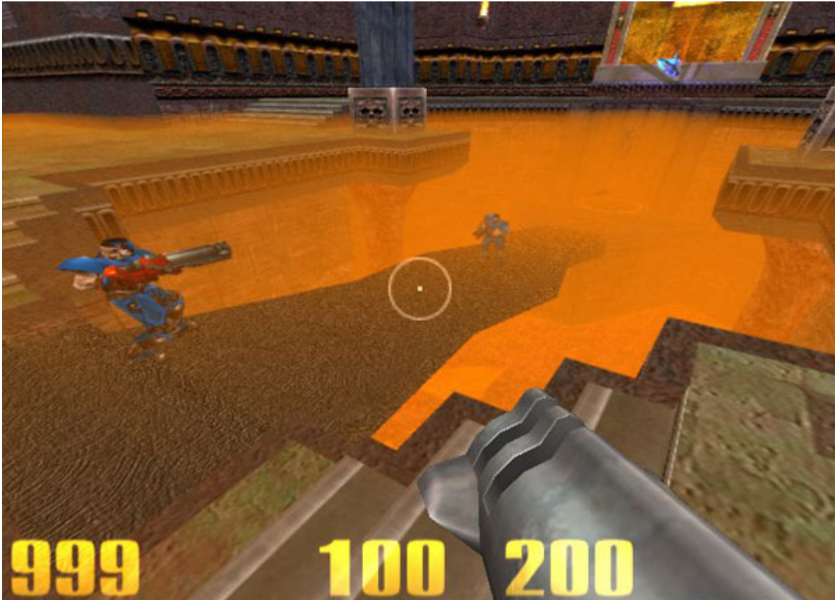
Fonts and crosshair layered over the ray traced image with semi-transparent quads in OpenGL
